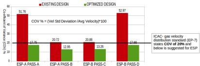
geometry modifications such as deflector plates, guide vanes, chamfer vanes are introduced. Based on customer preference, external duct geometry can also be modified for much better improvements in the flow. Multiple optimization cycles are carried out in order to arrive at a final
