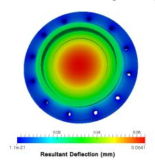
APH Bearing Housing is a major component which holds the whole weight of the APH. Bearing Housing is subjected to both axial and radial loads resulting from both weight of the APH & its operation. If the housing deflection exceeds 0.03 mm in the bearing outer race seating area, then it reduces the life of the bearing depending up on the deflection magnitude.
