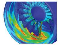
In the past few decades, FEA has become an indispensable tool within aerospace industry. The application of FEA within aerospace industry is widely spread into many areas. It is used towards solving problems like Structural analysis of various aerospace structures, Modal analysis, landing gear analysis, engine & nacelle component analysis, etc.
